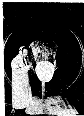
Fig. 35 Hypersonic structures model mounted in the Langley 8-foot high-temperature structures tunnel.
